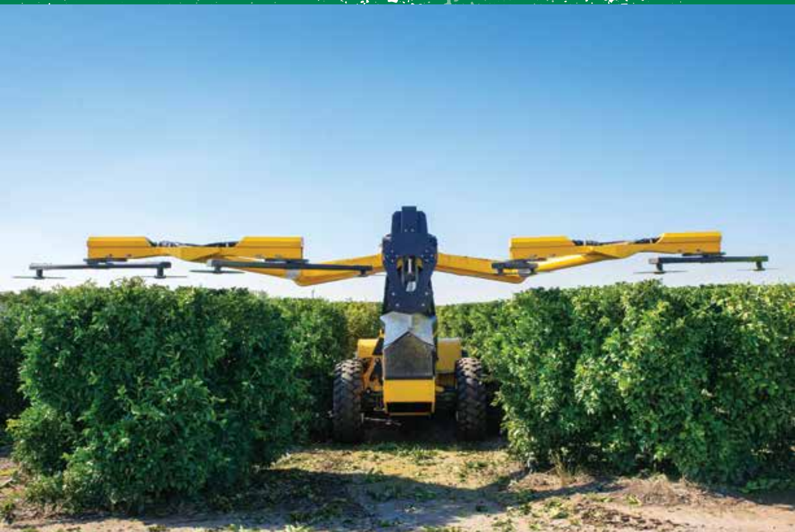
The HD1800RM hedges or tops both sides of an orchard row in a single pass.
