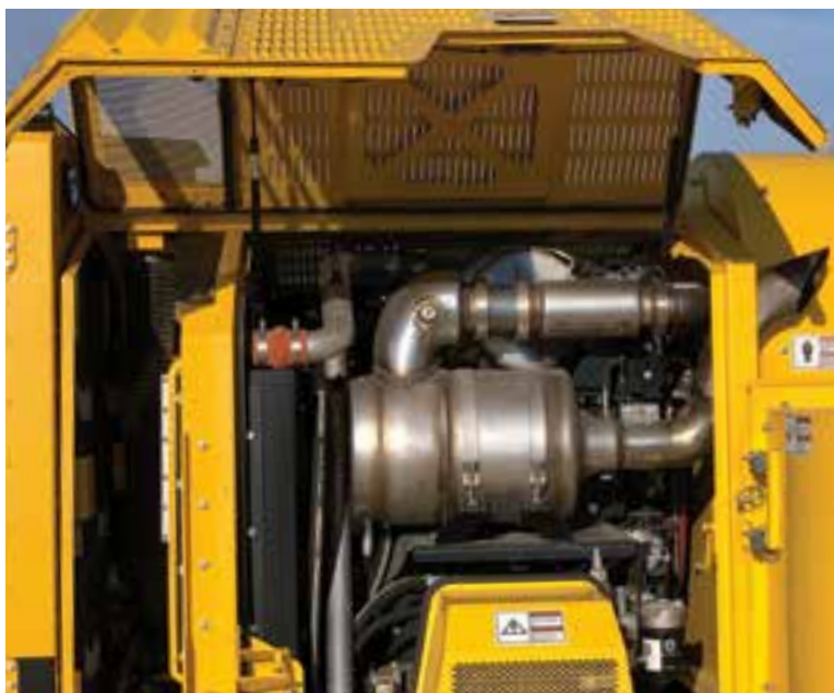
A custom PSL 4.5L engine fits the tight confines of the E7000 harvester.
