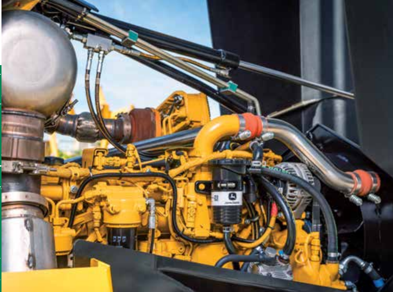
A 149-kW (200-hp) PowerTech™ PVS 6.8L engine and Funk Series 28000 pump drive power the drive system, saw blade, wing rotation, cylinder control system, and cooling system on the new TOL HD1800RM dual-boom hedger.
